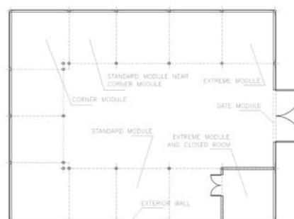
Figure 3. Plan of a typical cattle fold with 12 modules in U
