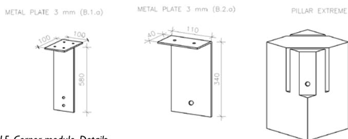
Figure 15. Corner module. Details
