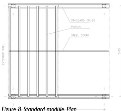
Figure 8. Standard module. Plan
