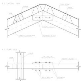
Figure 9. Standard module. Details of connections
