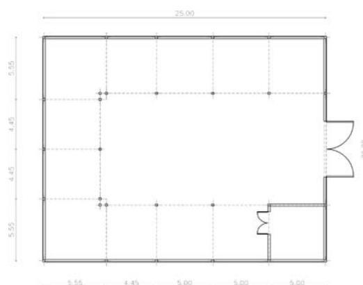
Figure 4. Plan of a typical cattle fold with 12 modules in U. Distances
